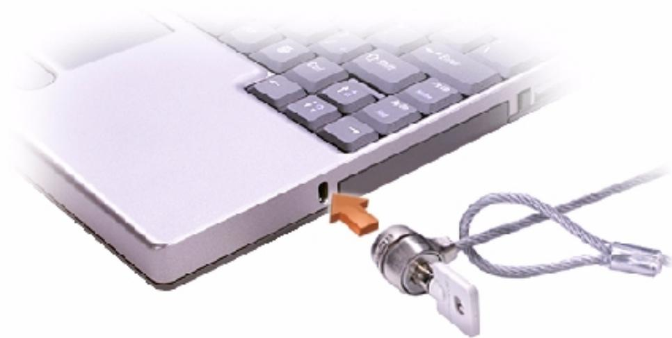
The slot lets you attach a commercially available antitheft device to the computer. Complete instructions for installing antitheft devices are usually included with the device.
